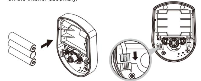
Match the interior assembly, the turnpiece should be vertical, and fasten the interior with screws.
