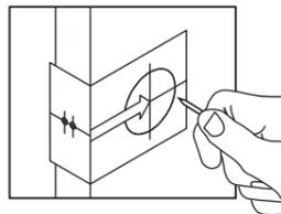
Select the height and backset as desired on the door face ; use the TEMPLATE as an indication to mark the center of the circle on the door face and the center of the door edge.
