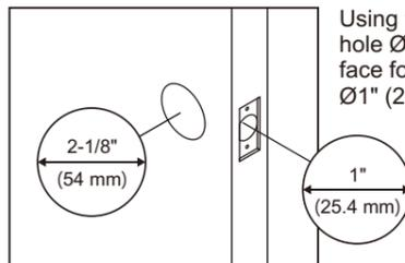
Using the marks as a guide to drill a hole Ø2-1/8" (54mm) through the door face for the lockset, then a hole of Ø1" (25.4mm) for latch.
