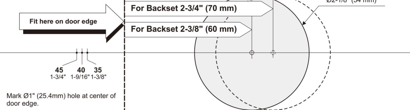
Mark Ø1" (25.4mm) hole at center of door edge.
